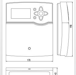
Inputs: 8 (9) inputs for Pt500, Pt1000 or KTY temperature sensors, 1 V40 impulse input, inputs for 2 digital Grundfos Direct Sensors<sup>™\*</sup>, 1 input for a CS10 irradiation sensor
